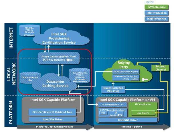
Figure 1: Intel® SGX DCAP Architecture Diagram
