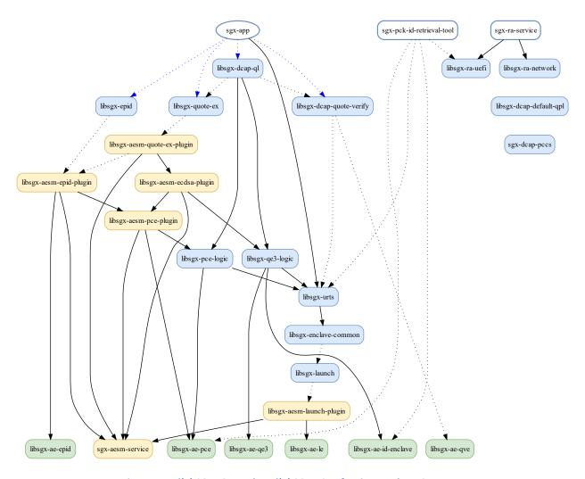
Figure 1 Intel(R) SGX PSW and Intel(R) SGX DCAP for Linux Package Structure
