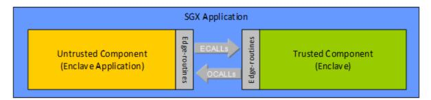
The first step in designing an Intel SGX enabled application is to identify the assets it needs to protect, the data structures where the assets are contained, and the set of code that operates on those data structures and then place them into a separate trusted library. Since the ISV knows the application best, the ISV should conduct a security analysis of the application and properly partition it making the decision about what code and data is placed in the enclave.
