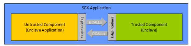
The first step in designing an Intel SGX enabled application is to identify the assets it needs to protect, the data structures where the assets are contained, and the set of code that operates on those data structures and then place them into a separate trusted library. Since the ISV knows the application best, the ISV should conduct a security analysis of the application and properly partition it making the decision about what code and data is placed in the enclave.
